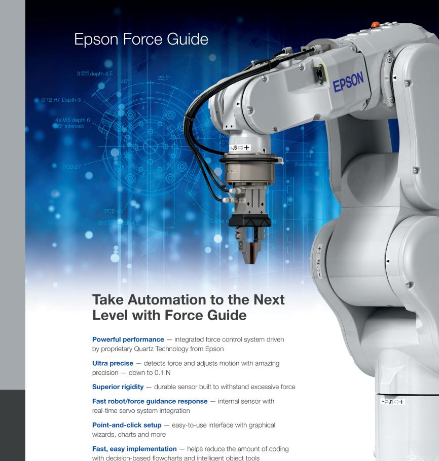
**Multi-axis force/torque sensor** — includes three linear and three
